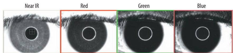
Figure 4. Multispectral imaging of a dark brown iris. The iris exhibits high iridal reflectance in the NIR channel. The reflectance decreases significantly in the other channels.
