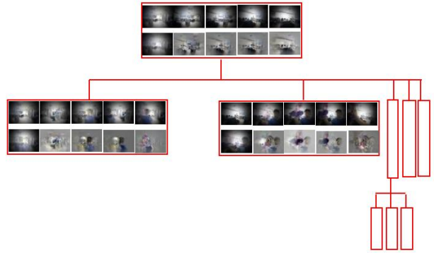
Figure 12: Tree Structure. Each block indicates a tree node. The first row of each node shows the x-cluster centers presented as images. The first image of the second row is the grand mean of all the x-clusters. The remaining images of the second row are the discriminating features represented as images. Here a Gaussian filter is used to alleviate noise.
