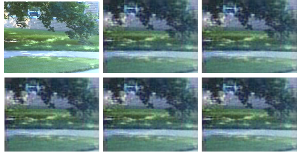
Figure 8: The reconstructed images from different levels. The first image is the original input image. Others are reconstructed images from Layer 1 to Layer 5 respectively.
